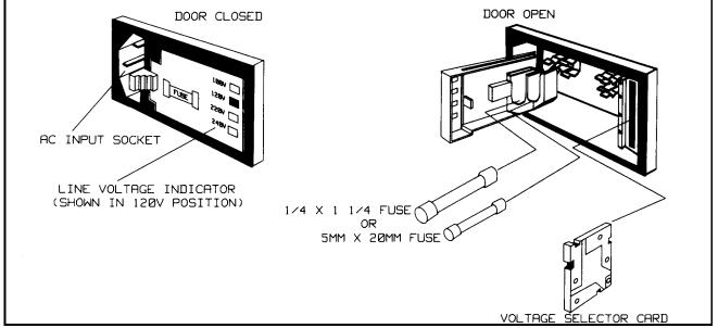
Figure 2-3. Line Module Detail
